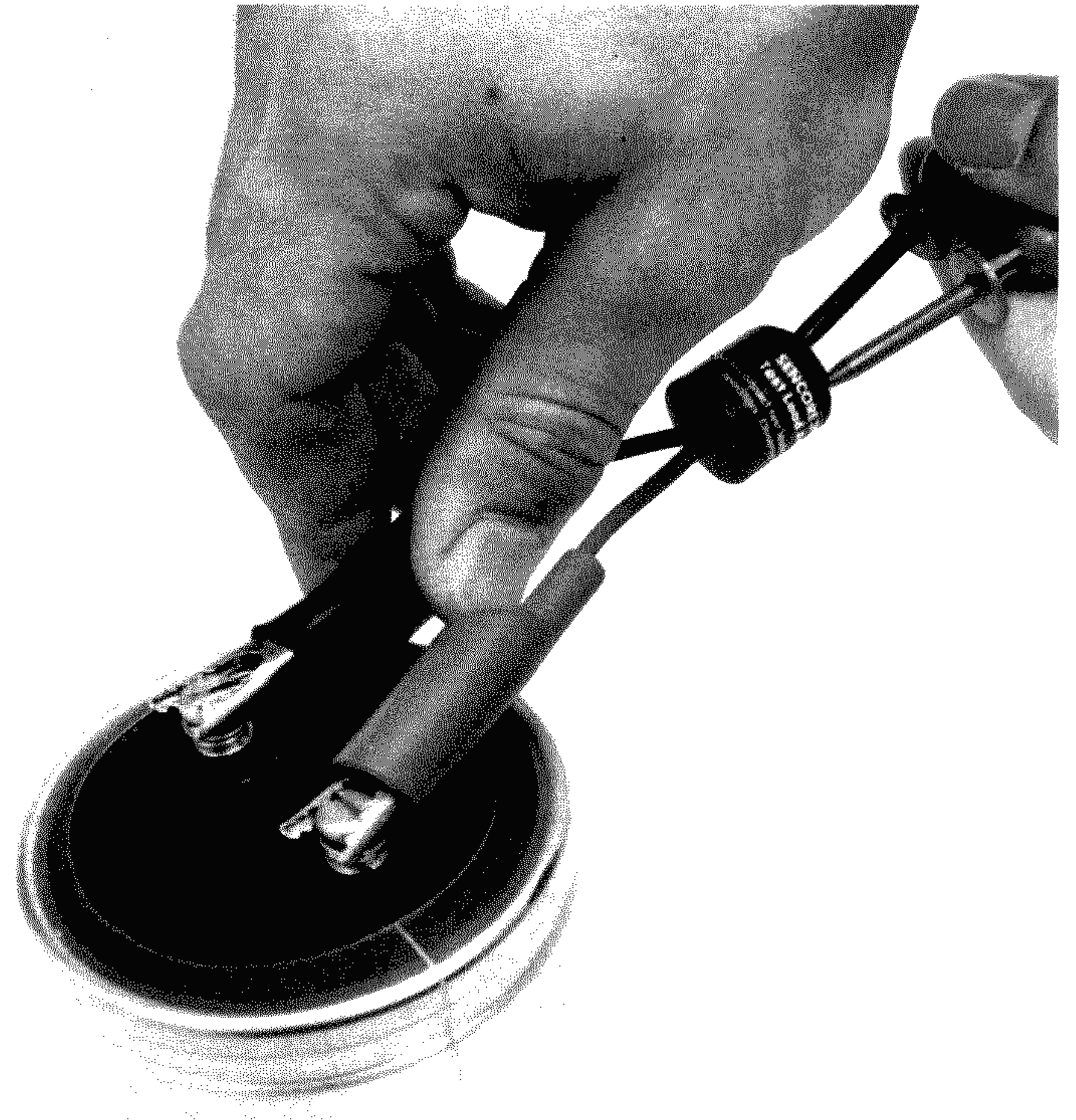
Fig. 10 - The 39G144 Test Lead Adapter allows large, screw-terminal capacitors to be connected to the LC102.
