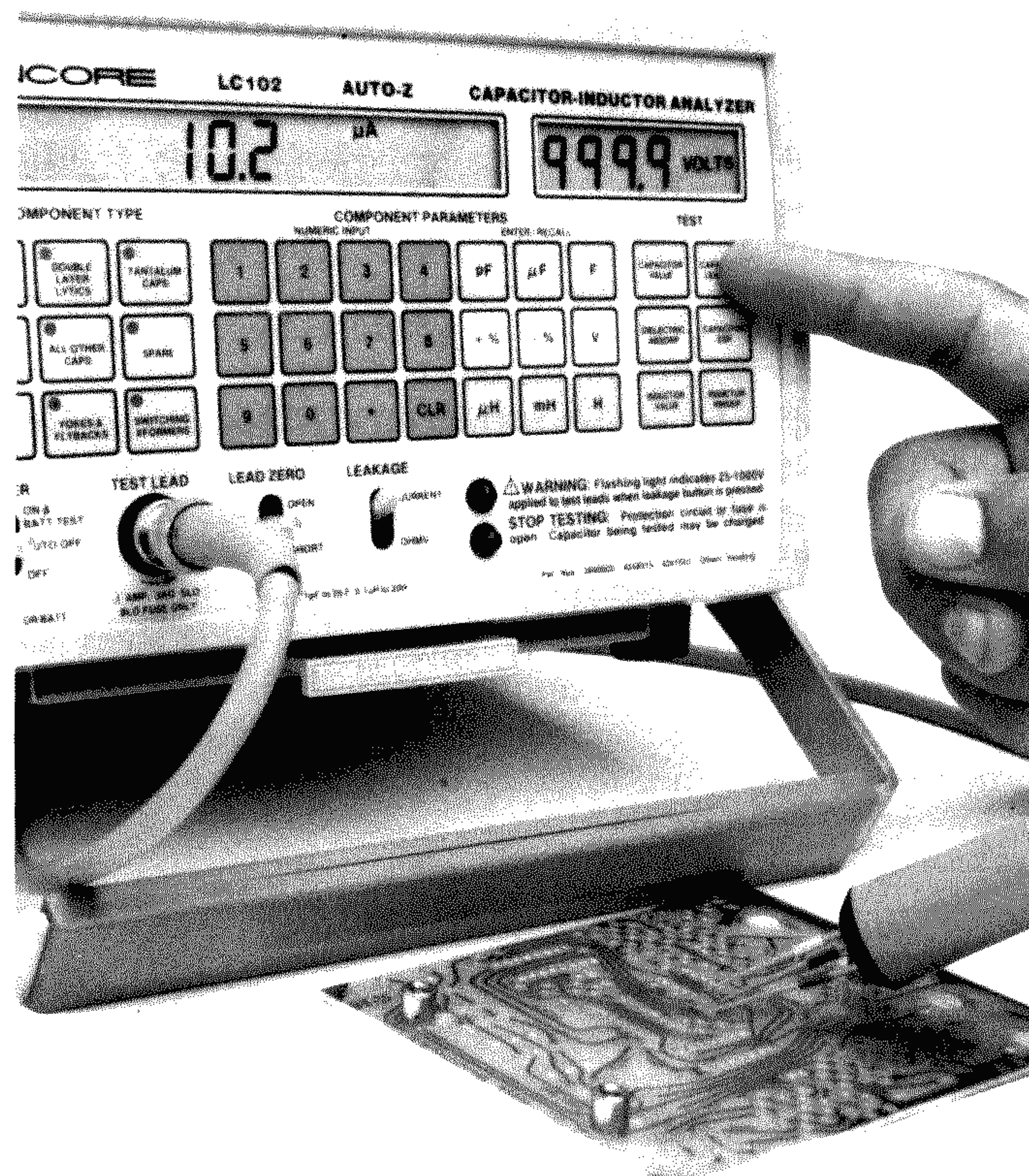
Fig. 65 - Small leakage paths can be detected with the LC102 Hi Pot test.
