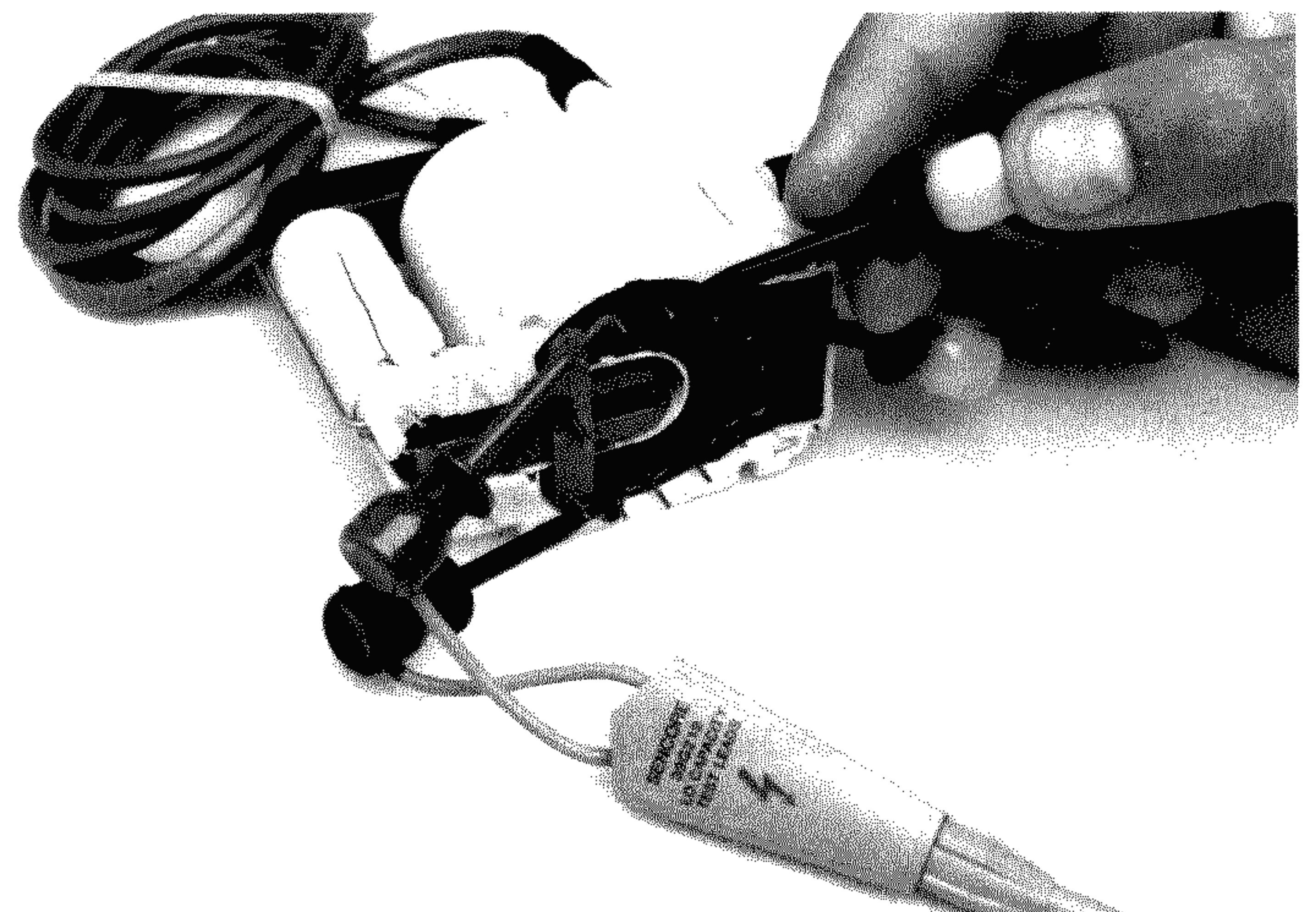
Fig. 61 — Use a jumper to determine if a flyback winding is open. An open winding will not cause the ringing test to change when a jumper is placed across it.
